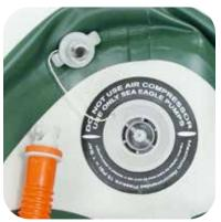
Screw hose with hook-in style adapter into pump handle and tighten. Firmly push adapter into valve. While pushing adapter firmly into valve, turn adapter to the right to lock it in valve. Note: red gasket may be very stiff at first. Stretch gasket to soften if it is too stiff to engage valve.
