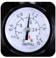
The pressure gauge will not begin to register until the board begins to get pressurized. Pump until the working pressure of between 12 and 15 PSI is reached.
