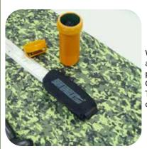
Wrap the carry handle pad around the carry handle. The pad can be found in the Orange Repair Kit cannister. The carry handle is a one-time installation.
