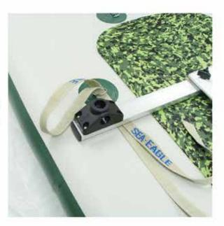
Slide the strap under the bar and over the rod holder base.
