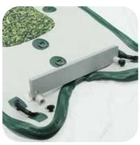
Insert motor mount board between the grommets. Put one washer on each long bolt and push through the grommets and board.
