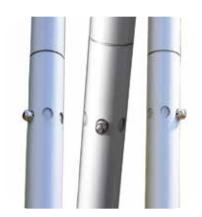
The additional holes in the shaft are for "feathering" the blades. Blades can be offset 45° from each other. This makes paddling into a stiff breeze easier as the blade that is not in the water will be able to slice through the wind with little resistance.
